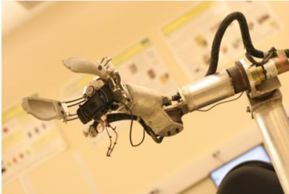
Figure 5.2: Camera and proximity sensor on gripper assembly
