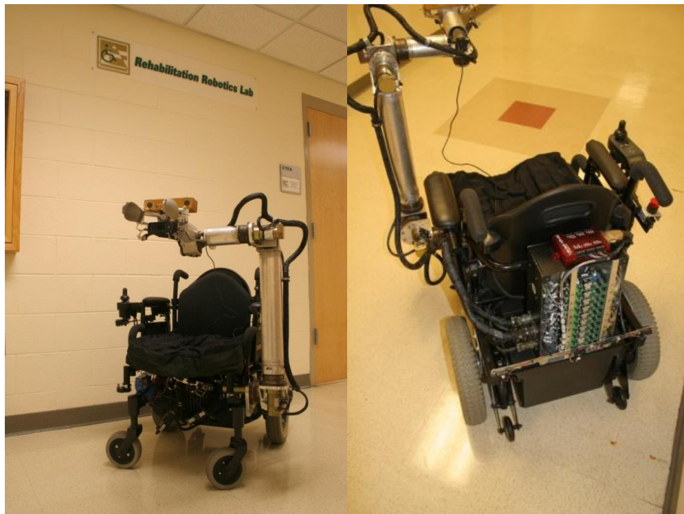
Figure 5.1: The 9-DoF WMRA system used for testing
