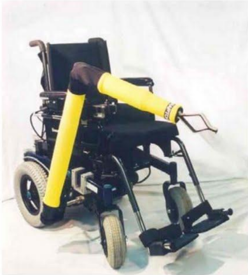
Figure 2.2: Applied Resources Raptor assistive arm (9)
