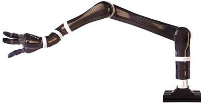
Figure 2.4: Kinova JACO assistive arm (11)
