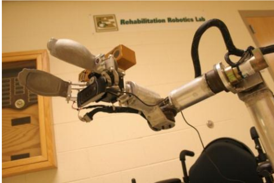
Figure 3.2: Stereoscopic camera on the WMRA
