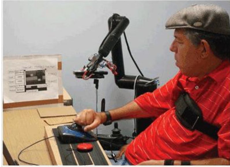
Figure 2.3: Exact Dynamics iARM assistive arm (10)
